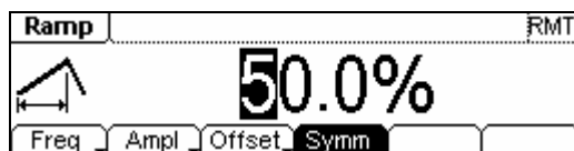
Figure 2-13 Ramp Signal Parameter Setting Interface
