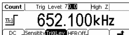
Figure 2-40 To set the coupling mode
