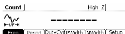
Figure 1-16 General interface of the counter
