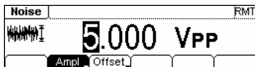
Figure 2-21 Noise Signal Parameter Setting Interface
