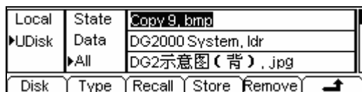
Figure 2-66 To use the USB Storage
