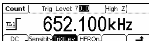
Figure 2-42 To set the trig level
