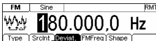
Figure 2-48 FM Waveform Parameter Setting Interface
