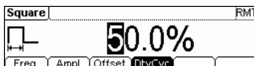
Figure 2-9 Square Signal Parameter Setting Interface
