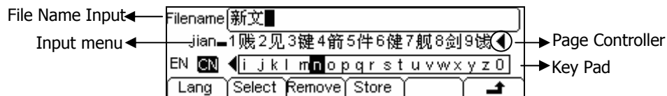
Figure 2-70 Chinese Input Interface
