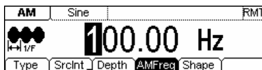
Figure 2-45 Modulated Waveform Parameters Interface for AM
