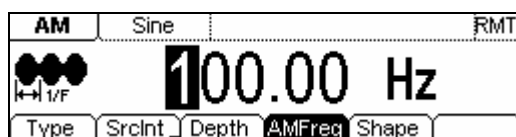
Figure 2-44 Modulated Waveform Parameters Interface
