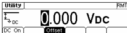
Figure 2-72 The DC Setting Interface
