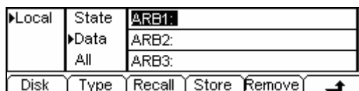
Figure 2-64 Save and Read Interface
