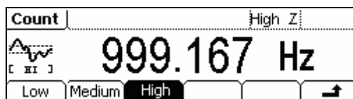
Figure 2-41 To set the sensitivity
